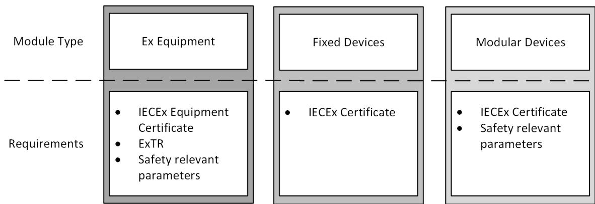
**Figure 2 – Requirements of a Modular Combination**
