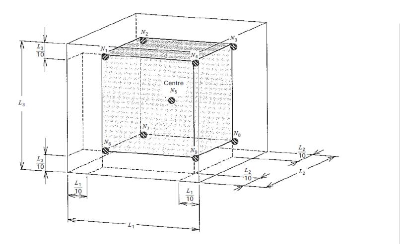
Above 2000 litres, six additional sensors on centre of each side
