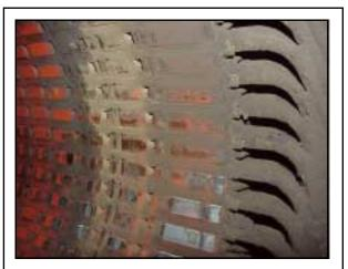
Figure 18. A minor stator core rub.
