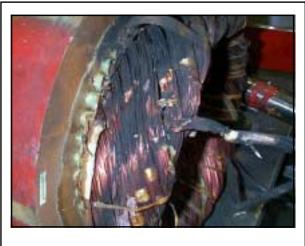
Figure 34. "Buried coils" in a lap winding.
