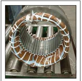
Figure 25. Typical concentric winding.
