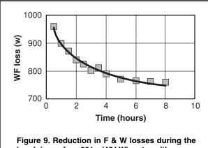
break-in run for a 60 hp (45 kW) motor with proper grease fill tested in the EASA/AEMT rewind study.
