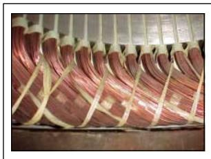
Figure 29. Coil extension for 4-pole motor as supplied by manufacturer.
