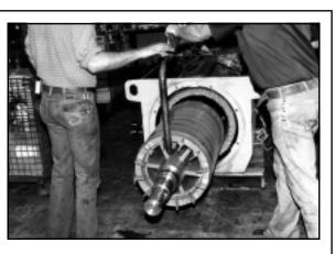
Figure 17. Rotor removal using a rotor removal tool.
