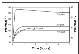
Figure 8. Short-term "break in" periods may not be adequate to reduce bearing losses, regardless of fill, as illustrated here. *From "Lubrication Fundamentals" by Mobil Oil Corp.*
