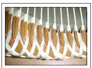
Figure 28. Typical coil extension for repaired 4-pole motor.
