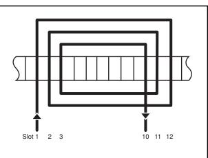
Figure 1. Coil group for 2-layer concentric winding. Coil pitch: 1-8, 10, 12 (spans 7, 9, 11)
