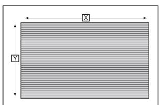
Figure 2. Lamination stack, above. Thermal conductivity is inhibited more in the perpendicular direction (Y) than the parallel direction (X) largely due to the interlaminar insulation and oxide coatings.
