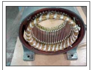
Figure 26. Typical lap winding.
