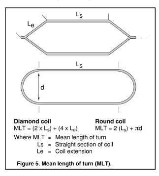
Avoid reducing the MLT too much. Doing so could make the stator difficult or even impossible to wind. It may even affect cooling, in extreme cases causing winding temperature to rise.
