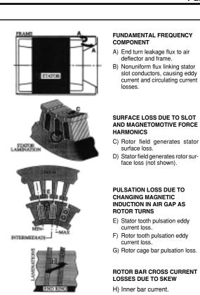
Figure 10. Components of stray loss.
