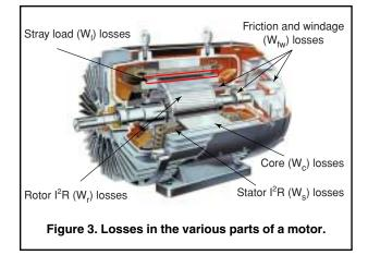
The core, friction and windage losses do not significantly change with motor load, provided the motor is operated from a fixed frequency. The I<sup>2</sup>R and stray load losses increase significantly as load is increased.
