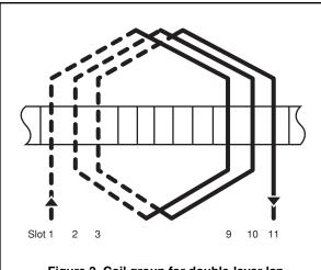
Figure 2. Coil group for double-layer lap. Winding short pitched 1-9 (span 8); dotted lines indicate coil sides in lower half of slot.
