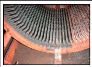
Figure 24. This core has been partially cleaned by using a high-pressure washer to remove the slot insulation debris.
