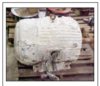
Figure 15. Motor with blocked cooling ribs.
