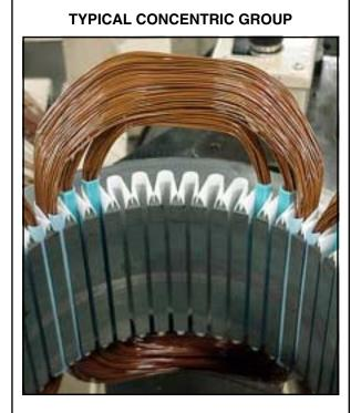
Figure 35. In a concentric winding, each coil has a different span. Each span has a different chord factor, making the effectiveness of each coil different.
