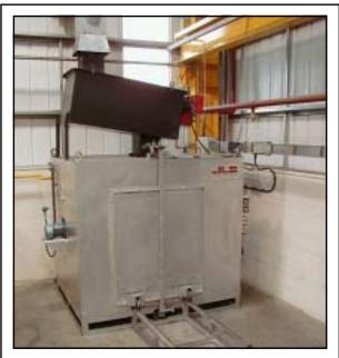
Figure 23. Controlled temperature burnout oven.
