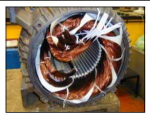
Figure 27. Inserting coils into a 2-pole stator
