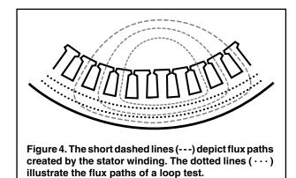
induced by the machine's winding, particularly when the rotor is removed (see Figure 4).
