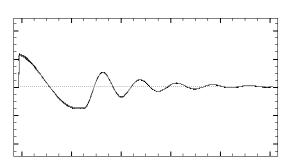
Figure 31. Satisfactory trace from phase balance/ surge comparison test.
