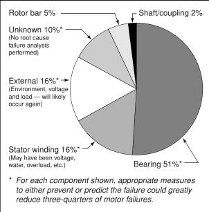
Figure 4. Failure by motor component.
