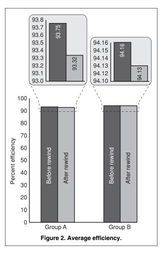
Group A) included control of core cleaning methods and rewind details such as turns/coil, mean length of turn, and conductor cross sectional area.
