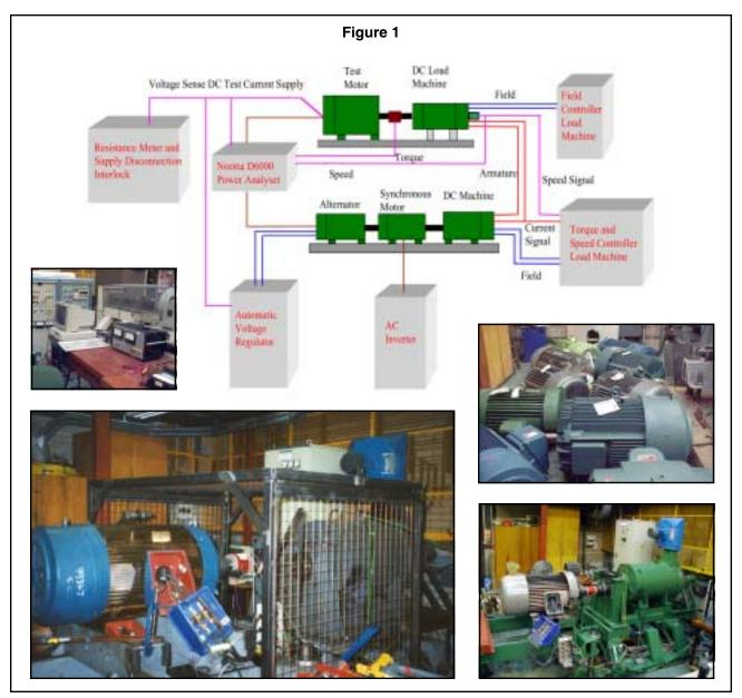
were measured before burnout and after stripping using a loop (ring) test and/or two commercial core loss testers.
