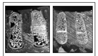
Figure 7. Increase slot fill from low (left) to the higher slot fill on the right. An increase in copper area reduces  $I^2R$  losses.
