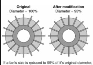
If a fan's size is reduced to 95% of it's original diameter, it will move (.95)<sup>5</sup> the volume of air it originally was able to move.
