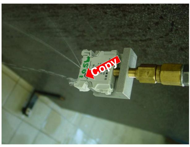
Static overpressure test with water according to IEC 60079 – 1
