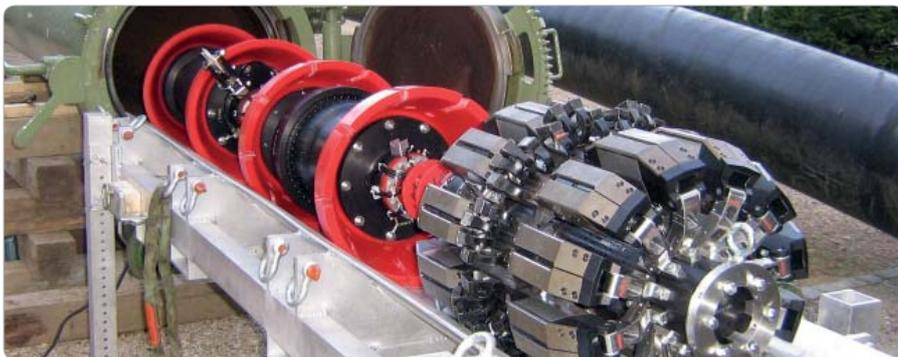
Smart pigging is carried in gas pipelines to measure thickness faults and dents (Photo: Gaznat)
