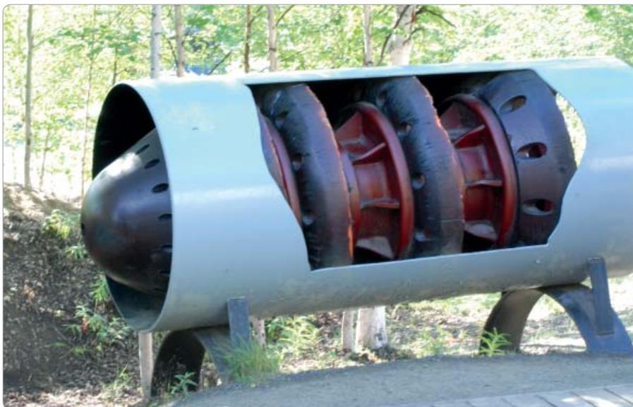
A pig on display in a section of cutaway pipe, from the Alaska Pipeline (Photo: Harvey Barrison, Wikimedia)
