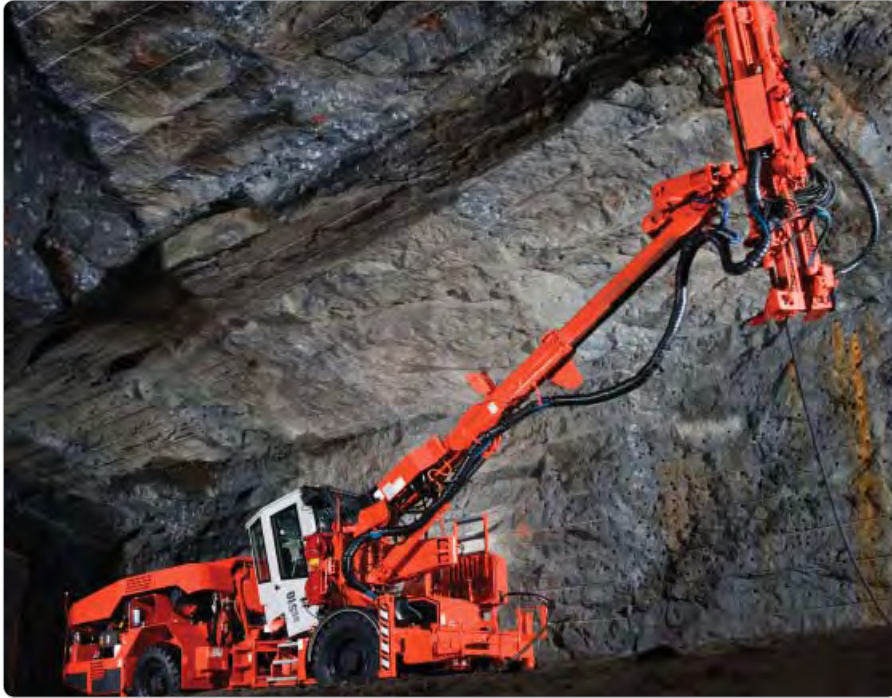
Modern roof bolters are automated to completely remove the risk of having the operator be exposed to falling rock while roof bolting is carried out
