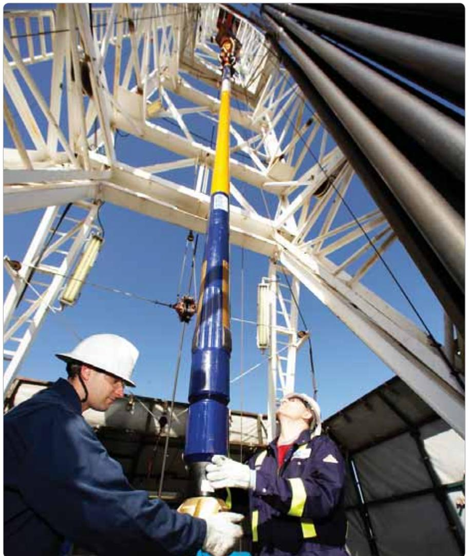
*Baker Hughes deploys an automated directional drilling assembly on a well in Canada (Photo: Baker Hughes)*
