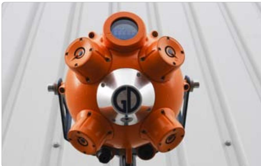
*Ultrasonic gas leak detector built to detect ultrasonic frequencies generated from pressurised gas leaks (Photo: a1-cbiss)*
