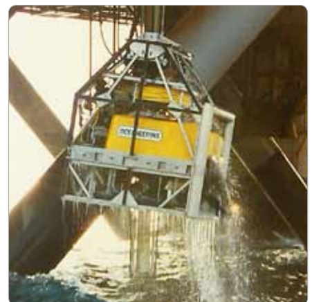
ROV lifted onto oil rig
