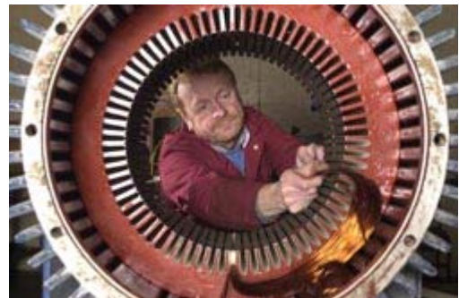
Overhaul of electrical rotating machinery
