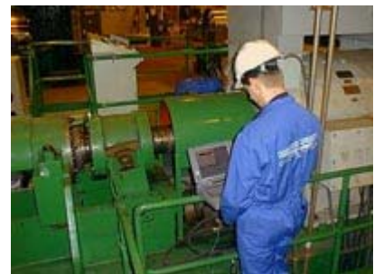
Vibration analyses on motors, signalling any deviations, are an extremely reliable method when used for monitoring bearing damage or wear.
