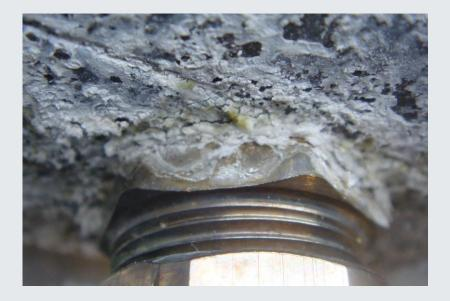
Brass gland fitted to an aluminium enclosure Superior Marine grade nickel plated brass gland fitted to an aluminium enclosure.
