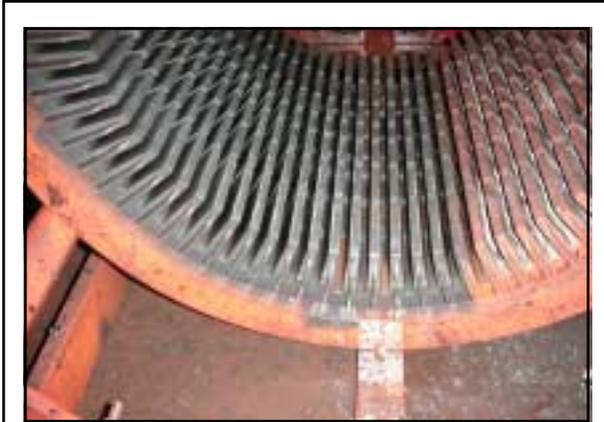
**Figure 24.** This core has been partially cleaned by using a high-pressure washer to remove the slot insulation debris.
