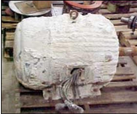
**Figure 15. Motor with blocked cooling ribs.**
