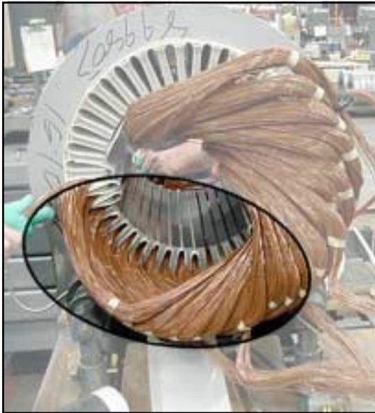
Figure 36. Lap winding showing all coils with the same span.
