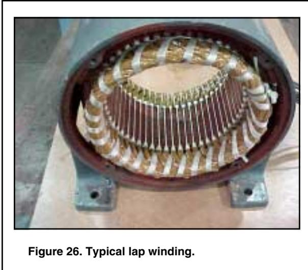
Figure 26. Typical lap winding.
