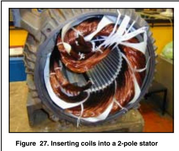
Figure 27. Inserting coils into a 2-pole stator
