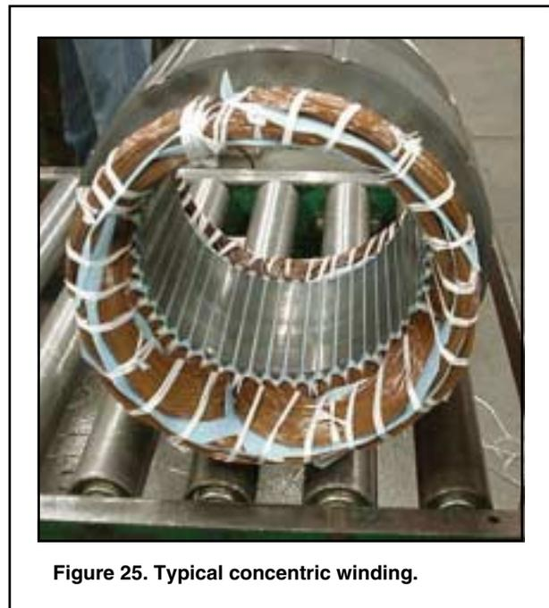
**Figure 25.** Typical concentric winding.
