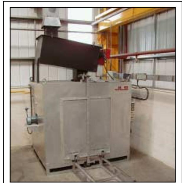
Figure 23. Controlled temperature burnout oven.
