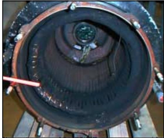
**Figure 21. Overall discoloration of the stator winding—usually indicates excessive temperature. Check load, power supply and cooling.**
