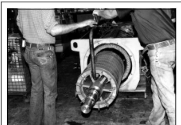
Figure 17. Rotor removal using a rotor removal tool.
