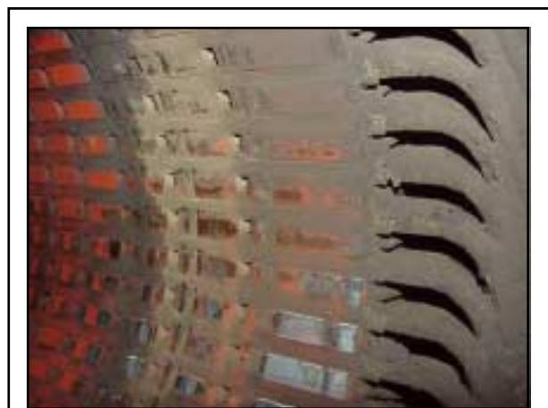
Figure 18. A minor stator core rub.
