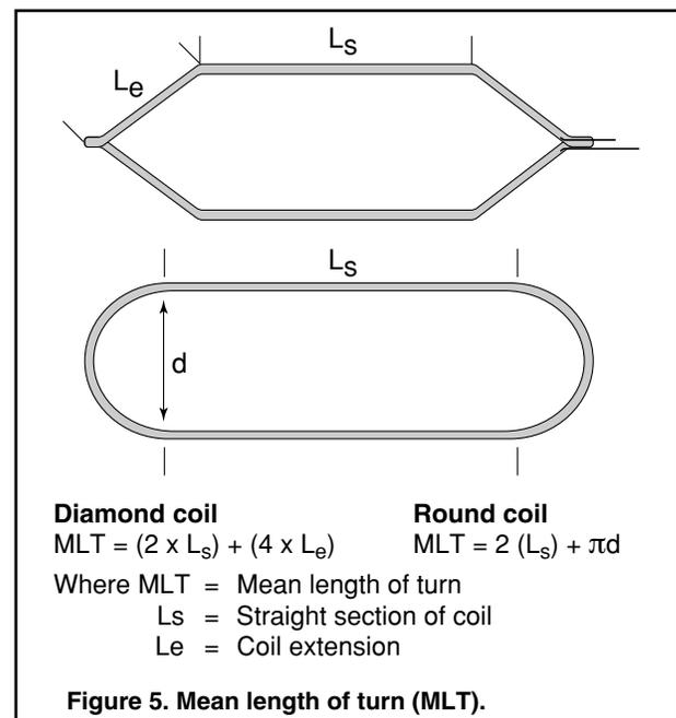
Avoid reducing the MLT too much. Doing so could make the stator difficult or even impossible to wind. It may even affect cooling, in extreme cases causing winding temperature to rise.
