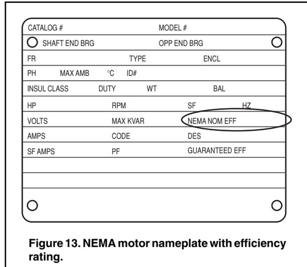
Figure 13. NEMA motor nameplate with efficiency rating.
