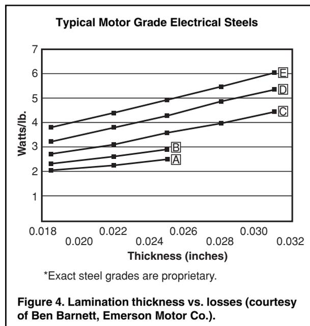
“Edge effects” caused by punching, however, and other factors mean that the eddy currents resulting from the induced voltages in the steel do not necessarily follow the same “square law” pattern. However, the “doubling approximation” is probably good enough for most practical purposes.
