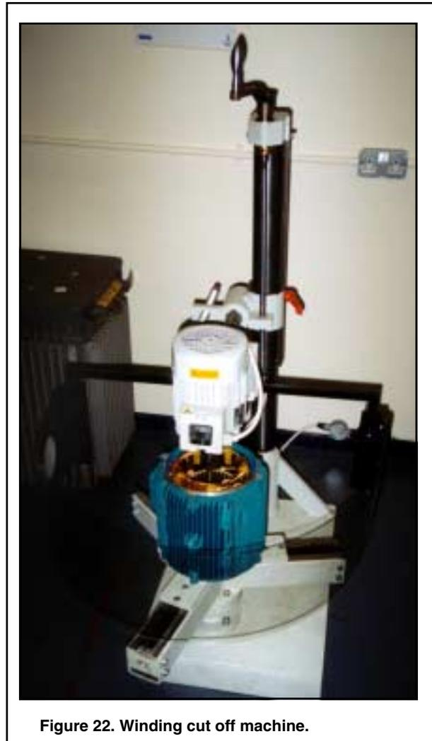
Figure 22. Winding cut off machine.
