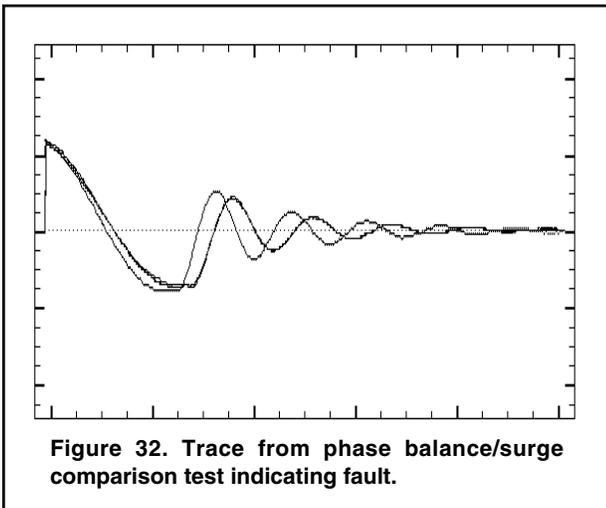
Figure 32. Trace from phase balance/surge comparison test indicating fault.
