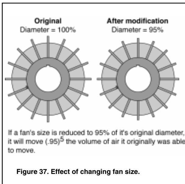
Replacing the original fan with a smaller fan of the same design is not recommended. Doing so will likely reduce air flow, causing the winding temperature to rise. That means increased losses and lower efficiency.
