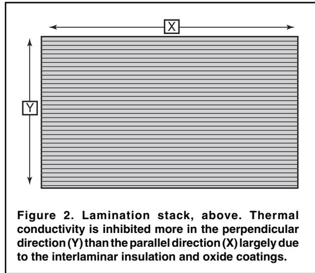
**Figure 2. Lamination stack, above. Thermal conductivity is inhibited more in the perpendicular direction (Y) than the parallel direction (X) largely due to the interlaminar insulation and oxide coatings.**
