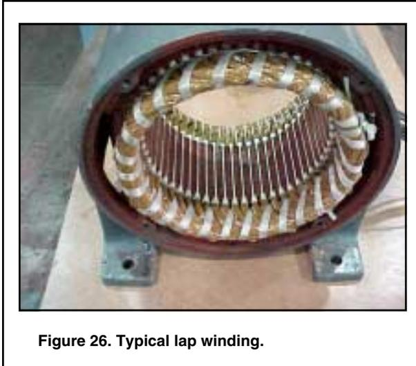
Figure 26. Typical lap winding.
