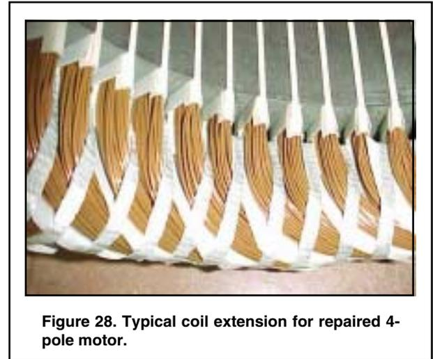
Figure 28. Typical coil extension for repaired 4-pole motor.
