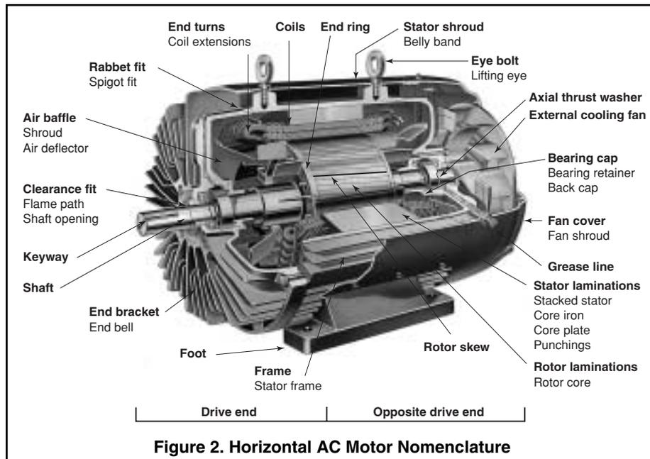
Figure 2. Horizontal AC Motor Nomenclature
