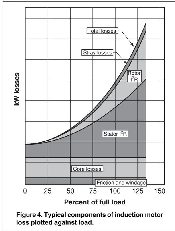
Figure 4. Typical components of induction motor loss plotted against load.
