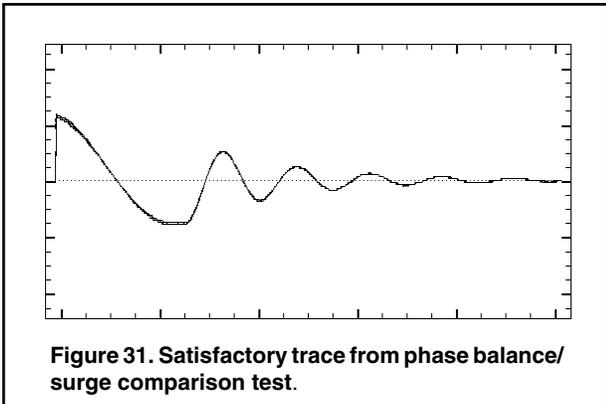
Figure 31. Satisfactory trace from phase balance/surge comparison test.
