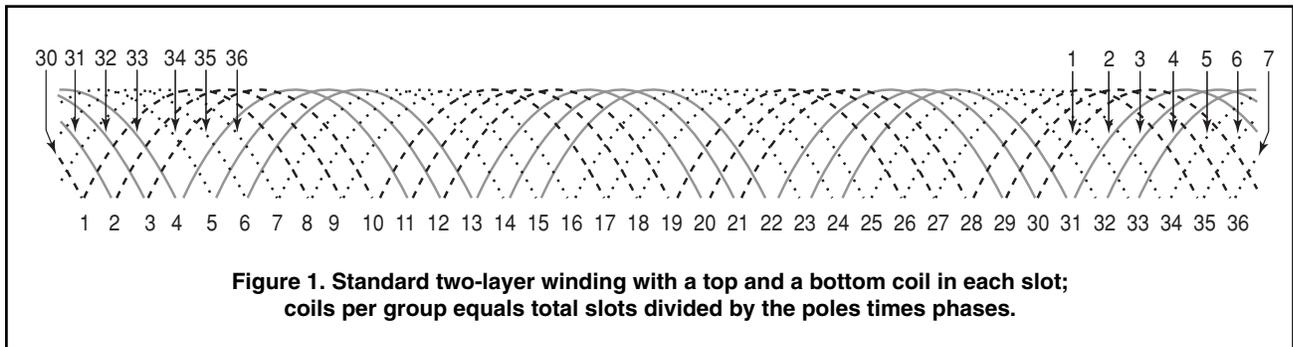
**Figure 1. Standard two-layer winding with a top and a bottom coil in each slot; coils per group equals total slots divided by the poles times phases.**
