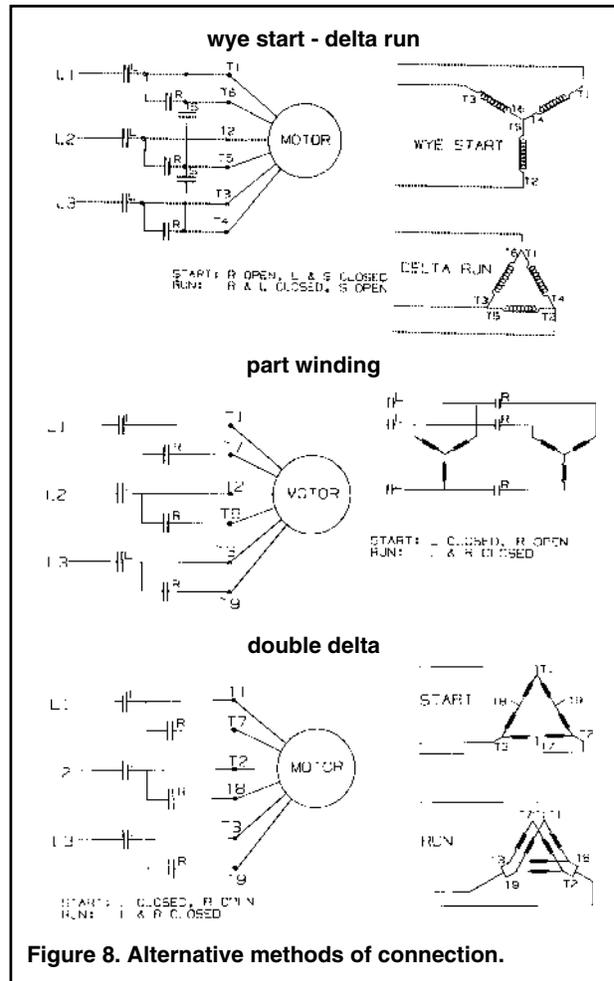
**Figure 8. Alternative methods of connection.**
