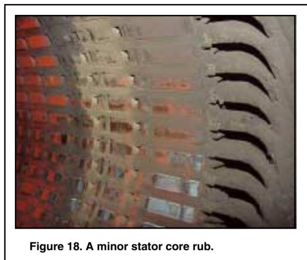
**Figure 18. A minor stator core rub.**
