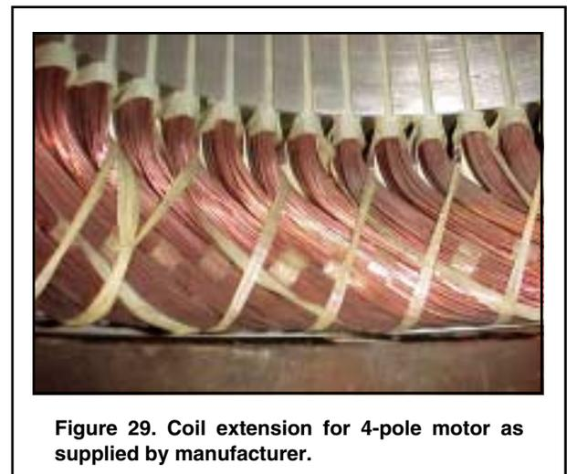
Figure 29. Coil extension for 4-pole motor as supplied by manufacturer.
