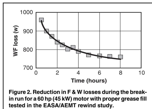
No change in lubrication was made on the rest of the motors in the test. As expected, bearing friction on the regreased motors increased and efficiency dropped 0.3 to 0.5 percent. Figure 2 illustrates the decrease in losses over time for a properly lubricated 60 hp (45 kW) motor in the EASA/AEMT study.
