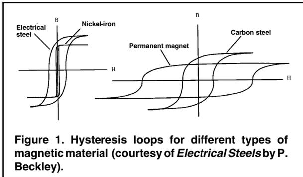
**Figure 1. Hysteresis loops for different types of magnetic material (courtesy of *Electrical Steels* by P. Beckley).**
