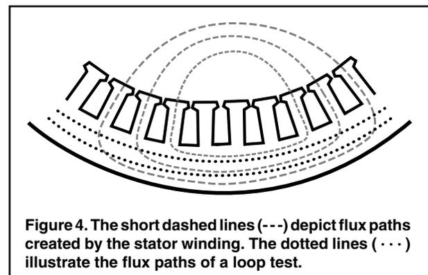
induced by the machine's winding, particularly when the rotor is removed (see Figure 4).
