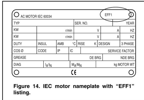
Figure 14. IEC motor nameplate with "EFF1" listing.
