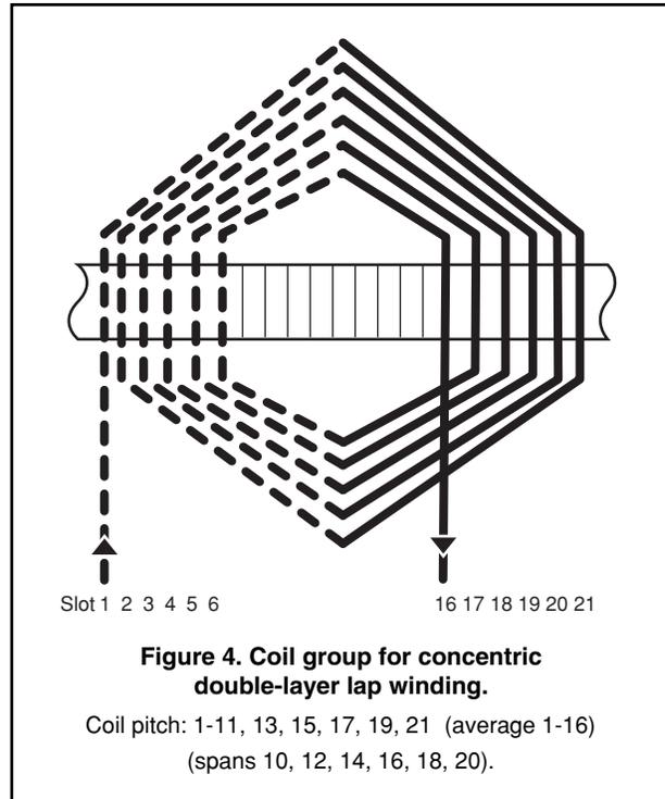
Figure 4. Coil group for concentric double-layer lap winding.
