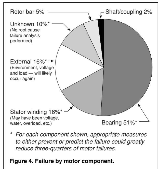
Figure 4. Failure by motor component.
