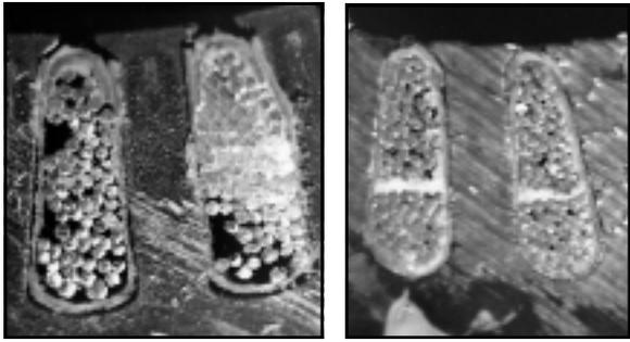
**Figure 7. Increase slot fill from low (left) to the higher slot fill on the right. An increase in copper area reduces I<sup>2</sup>R losses.**
