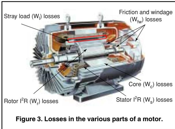
Figure 3. Losses in the various parts of a motor.
