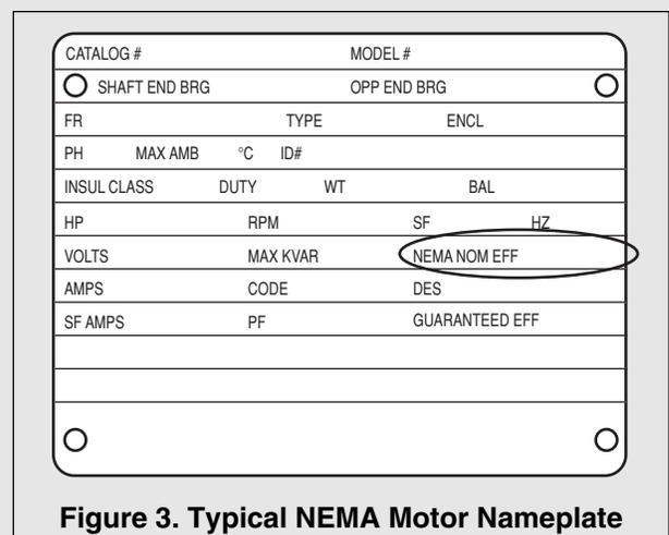
Figure 3. Typical NEMA Motor Nameplate
