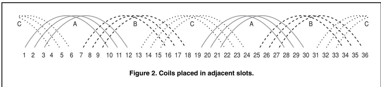
**Figure 2. Coils placed in adjacent slots.**
