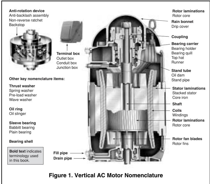
Figure 1. Vertical AC Motor Nomenclature
