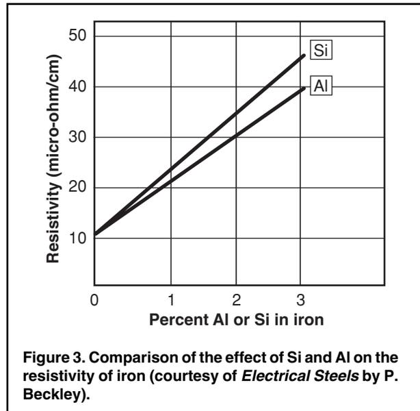
**Figure 3. Comparison of the effect of Si and Al on the resistivity of iron (courtesy of *Electrical Steels* by P. Beckley).**
