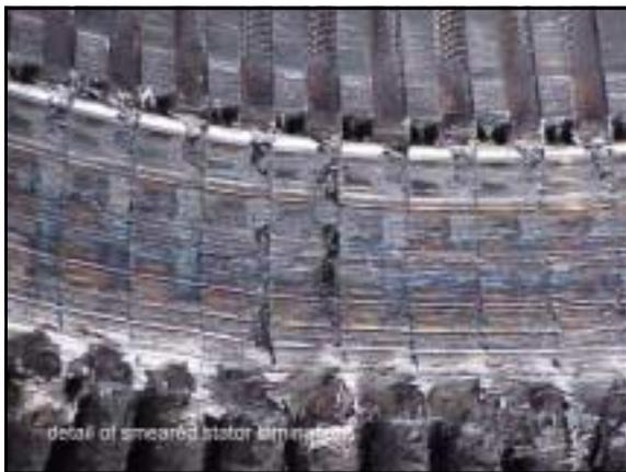
**Figure 20. Major mechanical damage to the stator bore; not repairable unless the core is restacked or replaced.**
