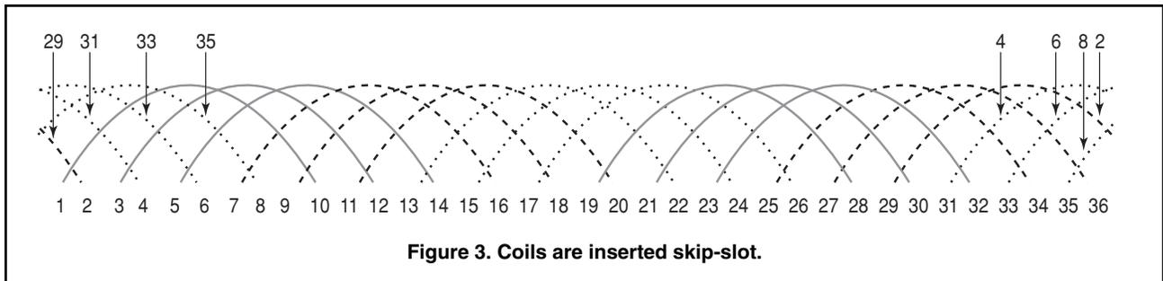
**Figure 3. Coils are inserted skip-slot.**
