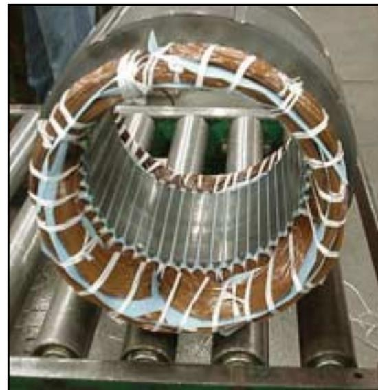
**Figure 25.** Typical concentric winding.
