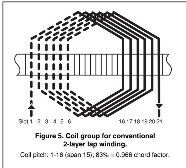
Figure 5. Coil group for conventional 2-layer lap winding.
