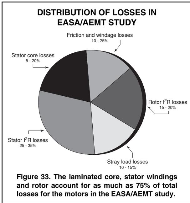
therefore, is to produce a motor that operates with minimal temperature rise. To achieve this, they address the areas where power is lost—to heat, friction or windage. They design longer stator cores, for instance, with correspondingly longer rotors or use better grades of electrical steel to decrease core losses. They also add more copper to windings (increase slot fill) to reduce copper losses.
