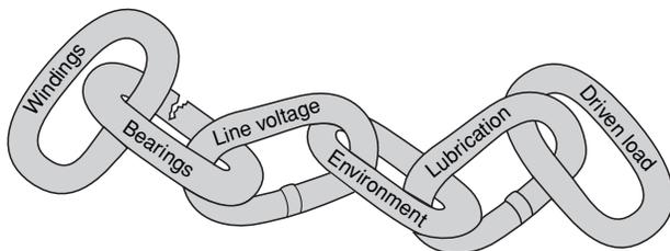
process, and to detect imminent failure before it occurs. Strengthening the weak link makes the entire process stronger. A motor subject to accidental wash-down should be of a suitable enclosure, and can be modified to further protect it from this hazard. Likewise, since more than 50% of electric motor failures start as bearing failures (Figure 4), bearing temperature detectors or vibration probes are logical options in many cases.
